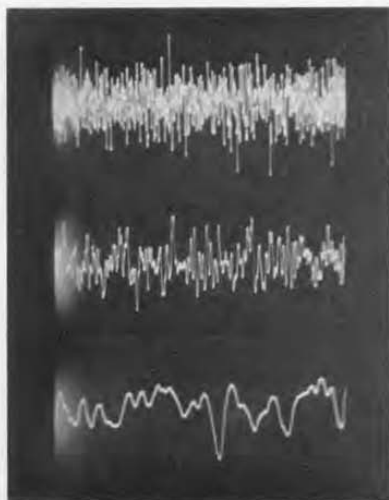
Figure 3. Oscillograms of three different samples of the output voltage wave of the noise generator. Only a single sweep and not a repetitive one was used in each case. The sweep speed for the middle trace was about four times that of the upper trace, and the wave was spread out even further in the lower trace by using a sweep speed of twenty times that of the upper trace.
